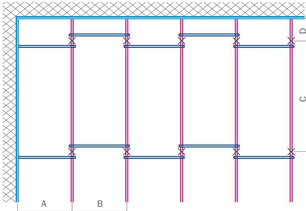
A = Max. 600/625 mm    B = Max. 600/625 mm    C = Max. 1500 mm    D = Max. 100 mm
